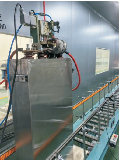
图12 铜条电极结构整机电感测量实物图 Fig. 12 Physical illustration of the complete device with copper strip electrode structure for inductance measurement
